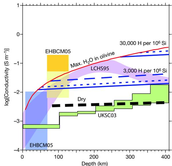
**Figure 2 | Comparison of laboratory data on electrical conductivity of hydrous olivine as a function of  $\text{H}_2\text{O}$  content with the geophysically observed electrical conductivity in the upper mantle beneath the Pacific.**
