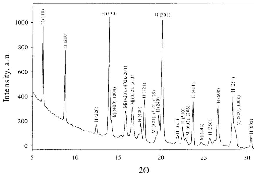
**Fig. 3.** Diffraction pattern obtained on a maskelynite of the Sixiangkou meteorite. Fifteen diffraction lines (H) are indexed in the hollandite structure (see Table 3). The remaining peaks (Mj) belong to the majorite-pyrox<sub>ss</sub> grains surrounding the maskelynite.
