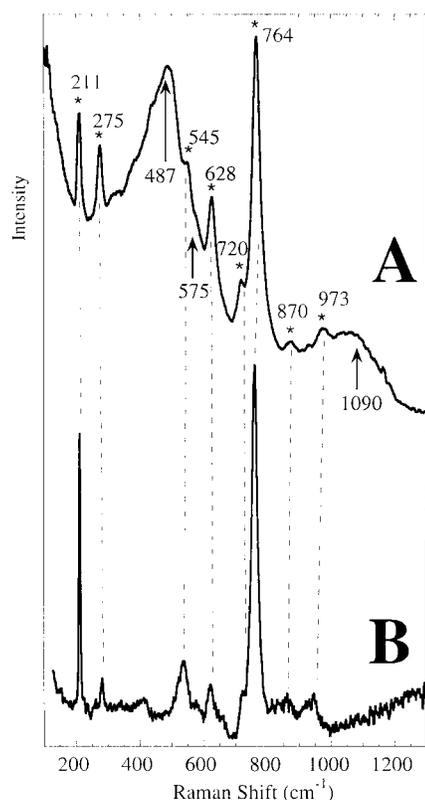
**Fig. 2.** (A) Typical Raman spectrum of the Sixiangkou maskelynites. The broad peaks (arrows) are close to those of  $\text{NaAlSi}_3\text{O}_8$  glass. The sharp peaks (asterisks) belong to hollandite. (B) Raman spectrum of  $\text{KAlSi}_3\text{O}_8$ -hollandite synthesized at 22 GPa and 1500 K. The sharp peaks of the spectrum in (A) correspond within a few wave numbers to those of  $\text{KAlSi}_3\text{O}_8$ -hollandite.
