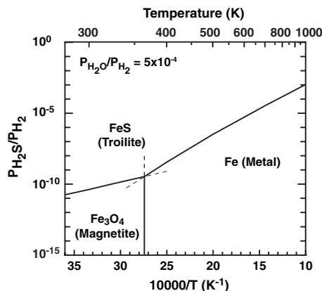
**Fig. 4.** Calculated equilibrium temperatures for Fe-metal, troilite ( $\text{FeS}$ ) and magnetite ( $\text{Fe}_3\text{O}_4$ ) as a function of  $P_{\text{H}_2\text{S}}/P_{\text{H}_2}$  ratio. The magnetite phase boundary is calculated assuming canonical solar nebular  $\text{H}_2\text{O}/\text{H}_2$  ratio of  $5 \times 10^{-4}$  (30). Magnetite is considered as a proxy of a new-PCP. Thermodynamic data from JANAF tables (31) were used for calculations.
