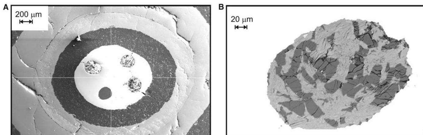
**Fig. 1.** Back-scattered electron images of sample capsules. **(A)** A radial section through the high-pressure assembly shows the outer pressure medium and furnace with an inner four-chamber Re capsule (white). Three sample chambers contain garnet and Ca-perovskite assemblages (which appear lighter), whereas
