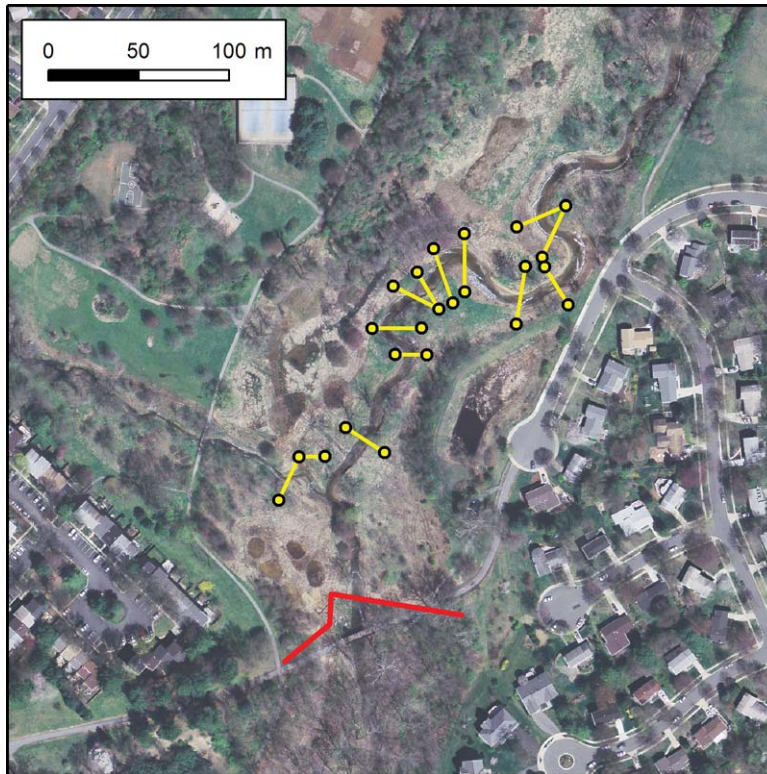
Figure S4. Here we show that stream channel erosion and migration monitored for 41 years (yellow lines with end points mark approximate locations of surveyed cross sections) in a study of meander migration and floodplain formation near the headwaters of Watts Branch, MD ( S12 , S13 ) are located immediately upstream of a breached 19th c. mill dam (red line marks approximate location) that was not recognized by previous workers. (Flow is from top to bottom, approximately north to south, in view.) This dam supplied water to Wootton's Mill, which operated until 1905 and was located <1 km downstream of the dam (toward bottom of view). The higher valley flat surface upstream of the dam is interpreted here as a fill terrace rather than as a floodplain, even though it might now receive occasional overbank flow.
