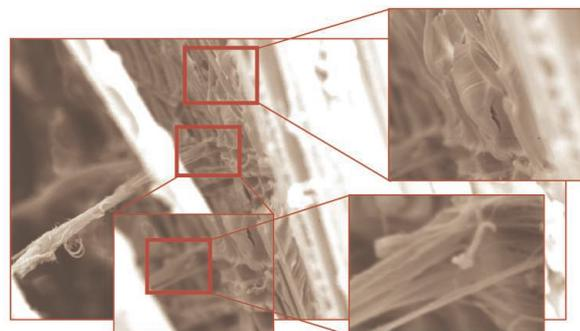
**A pathway to supernanocomposites?** (Left) Advanced laminated composite with nanofiber-reinforced interfacial layer. (Right) In situ observation of interlaminar toughening nanomechanisms including Velcro-like crack bridging by nanofibers.
