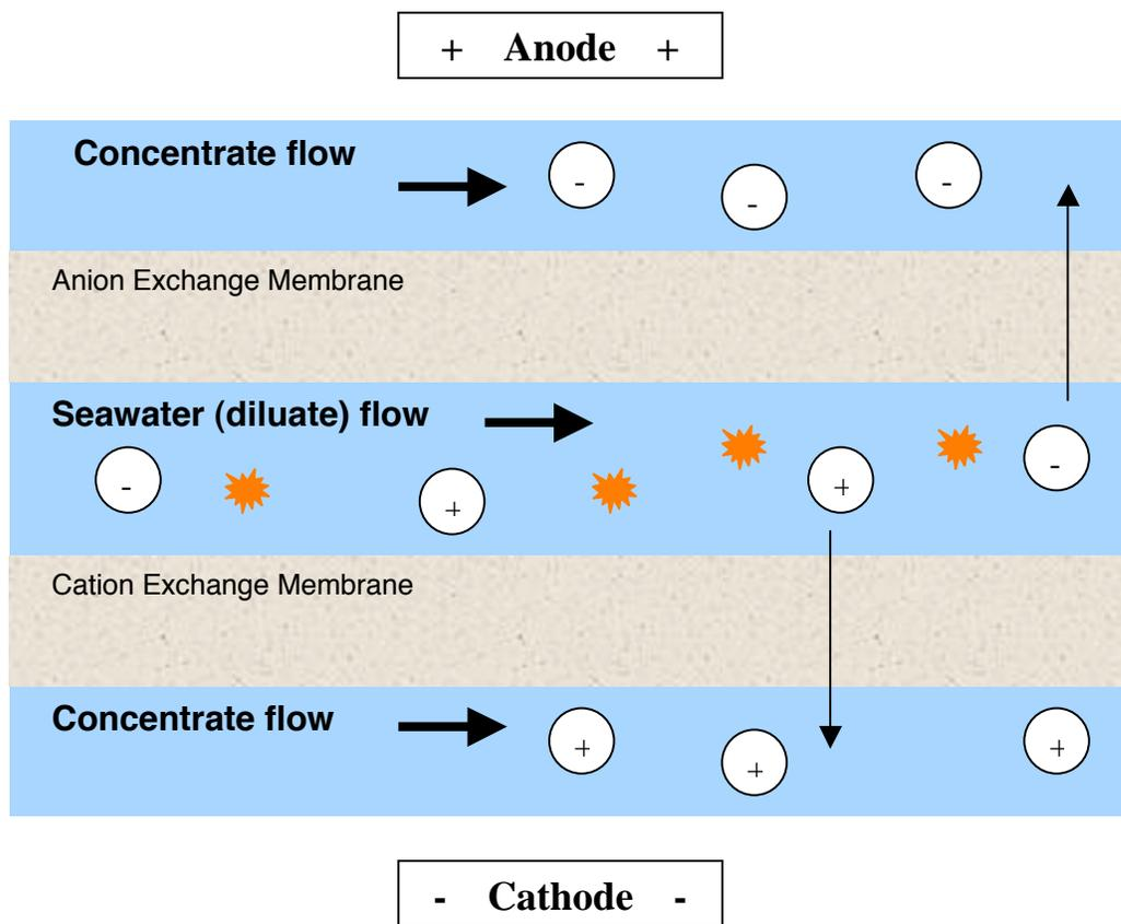
**Fig. S9.** Electrodialysis. Seawater contacts a concentrate flow across many pairs of anion/cation exchange membranes through which a DC current is directed. In this process, ions move from the seawater flow (diluate) into the concentrate flow, while dissolved molecules (orange globules) are retained in the diluate flow. Dissolved molecules in the salt-free diluate flow are subsequently concentrated using reverse osmosis.
