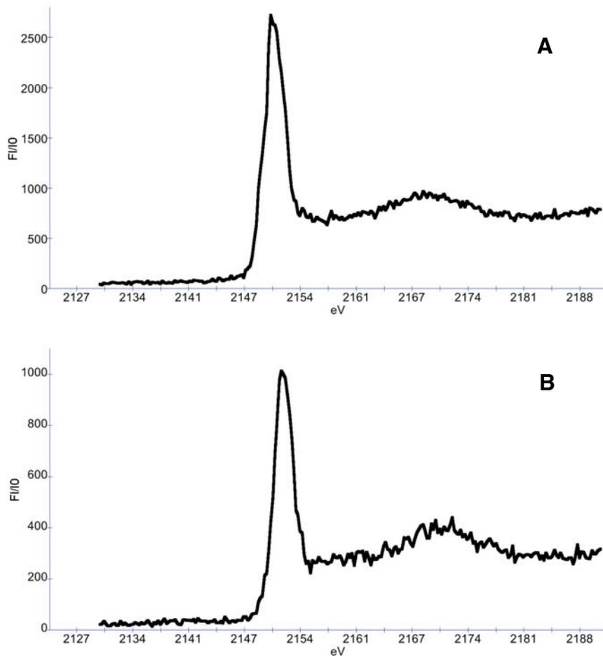
**Fig. S8.** X-ray fluorescence spectra of standard biogenic polyphosphate. These phosphorus X-ray fluorescence spectra were collected from intracellular polyphosphate granules of the freshwater algae: (A) *Chlamydomonas* sp. and (B) *Chlorella* sp. As shown in these spectra, biogenic polyphosphate yields phosphorus fluorescence spectra characterized by a featureless primary peak and a single high-energy peak located 18eV above the primary peak position.
