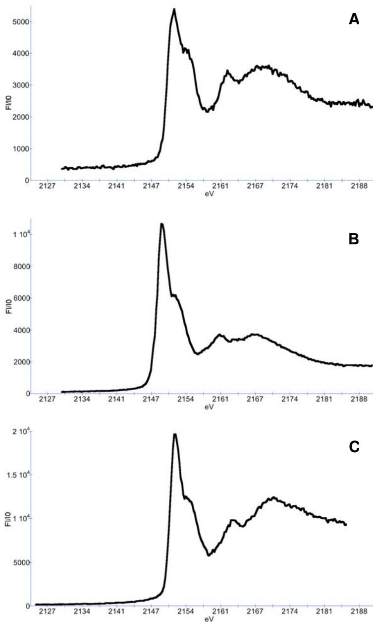
**Fig. S7.** X-ray fluorescence spectra of standard calcium phosphate mineral phases. Normalized phosphorus X-ray fluorescence spectra of (A) carbonate fluorapatite, (B) hydroxyapatite, and (C) phosphorite are all characterized by a primary peak “shoulder” and two high-energy peaks located at 11eV and 18eV above the primary peak position. Based on our analyses, other calcium phosphate minerals yield subtly different yet distinct phosphorus X-ray fluorescence spectra.
