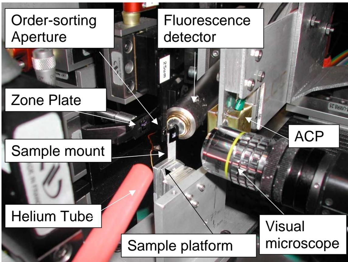
**Fig. S6.** Instrument set-up at beamline 2-ID-B. Analyses are performed with multiple X-ray detectors and optical components positioned at millimeter to centimeter distances away from the sample. Instruments are moved using high spatial resolution motors. See text for a description of instrument components. Photo courtesy of Juergen Thieme.
