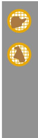
**Fig. S5.** SXM Sample Mount. Carbon/formvar-backed copper TEM grids (3mm diameter; Ted Pella™) were attached to the upper and lower holes of aluminum mounting sticks. Milligrams of sediment were deposited onto the TEM grids.
